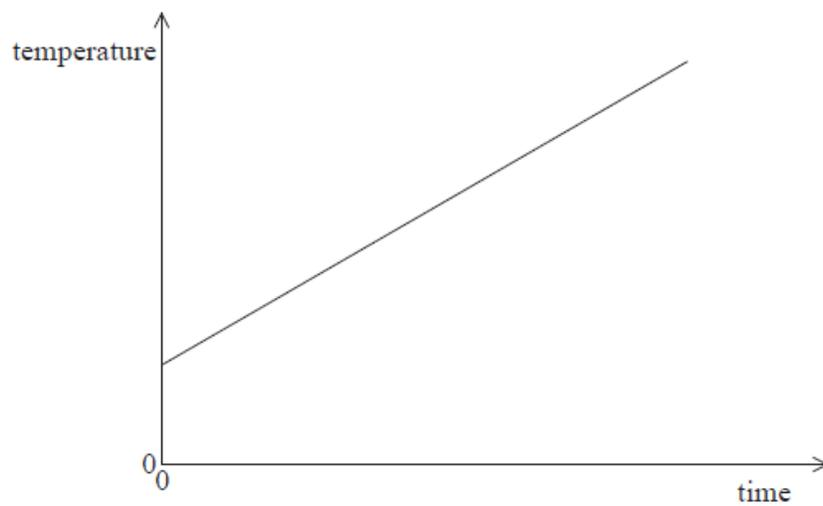
The gradient of the graph is  $k$  and no energy is lost to the surroundings. What is the power of the heater?
