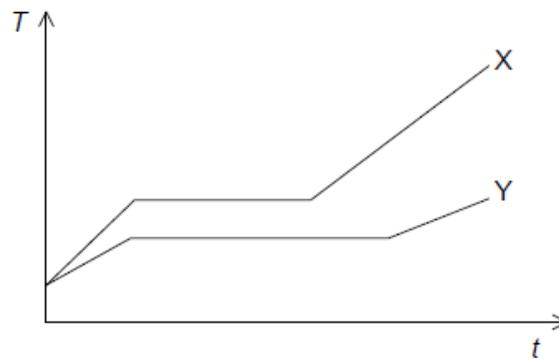
What is the correct comparison of the specific latent heats  $L_X$  and  $L_Y$  and specific heat capacities in the liquid phase  $c_X$  and  $c_Y$  of X and Y?
