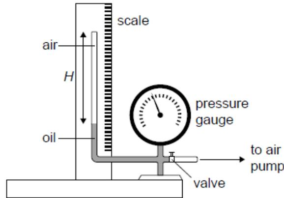
The pump forces oil to move up the tube decreasing the volume of the trapped air.
