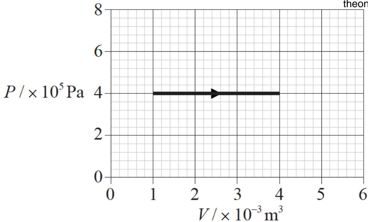
The change in the internal energy of the gas during this expansion is 1800 J. What is the amount and the direction of thermal energy transferred?
