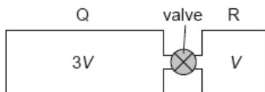
The valve is opened in such a way that the temperature of the gases does not change. What is the change of pressure in Q?
