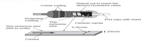
The wire used in such a resistor has a rectangular cross-section as shown. Determine the length of nichrome wire required to make a  $2.0\,\mathrm{k}\Omega$  resistor. [Resistivity of nichrome =  $1.20\,\times\,10^{-6}\,\mathrm{m}$ ] [2]
