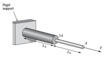
(i) Show that the total extension,  $\Delta x_{\rm total}$ , of the bar under the action of an applied force, F, as shown in the diagram, can be given by:
