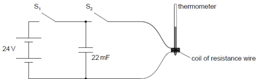
A power supply of emf (electromotive force)  $24 \text{ V}$  and of negligible internal resistance is connected to a capacitor and to a coil of resistance wire using an arrangement of two switches. Switch  $S_1$  is closed and, a few seconds later, opened. Then switch  $S_2$  is closed.
