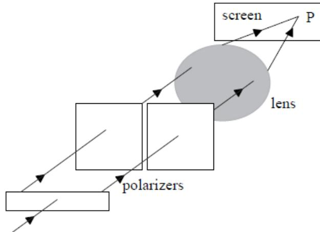
A lens brings the light to focus at point P on a screen. The lens does not introduce any additional path difference.
