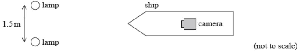
The camera has a circular aperture of diameter 6.2 mm. The lamps are separated by 1.5 m. Determine the maximum distance between the camera and the lamps at which the images of the lamps can be distinguished.
