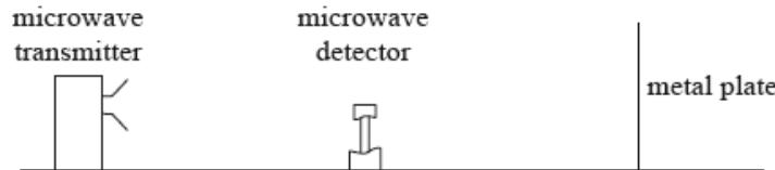
A microwave detector is moved along a line normal to the microwave transmitter and the metal plate. The detector records a sequence of equally spaced maxima and minima of intensity.
