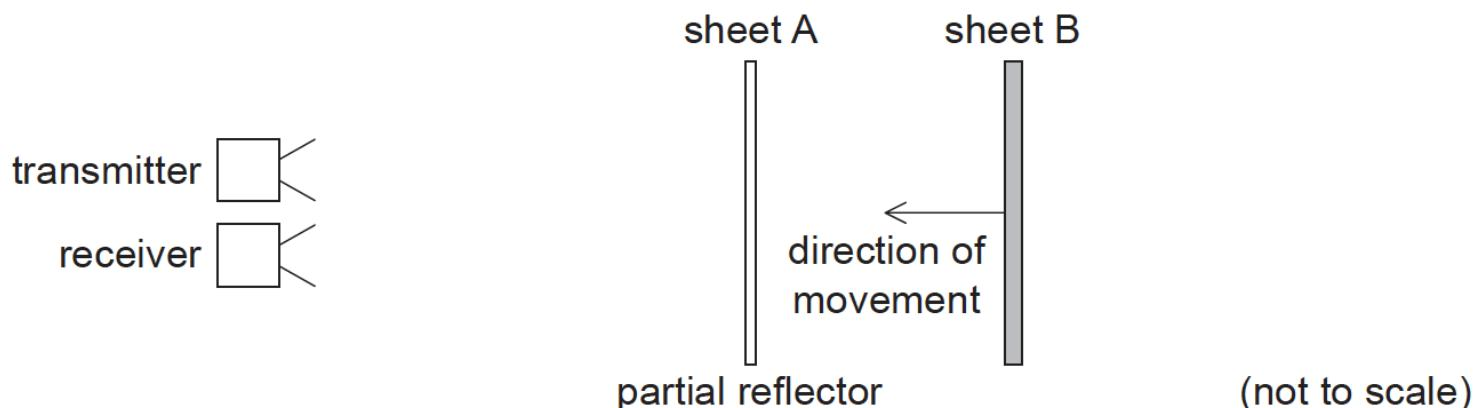
Sheet A is fixed and sheet B is moved towards it. While sheet B is moving, the intensity of the signal detected at the receiver goes through a series of values.
