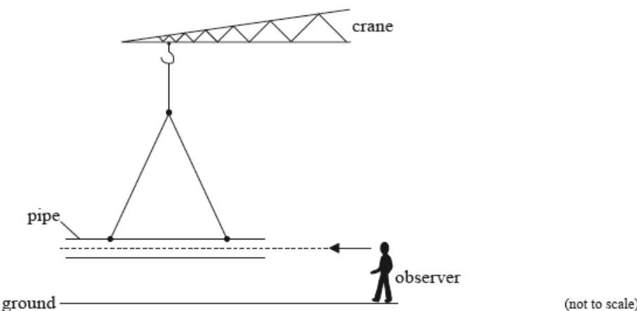
Wind blows across one end of the pipe. This causes a standing wave to form in the air of the pipe, producing the first harmonic. The pipe has a length of 2.1 m and the speed of sound in air is  $330 \text{ m s}^{-1}$ .
