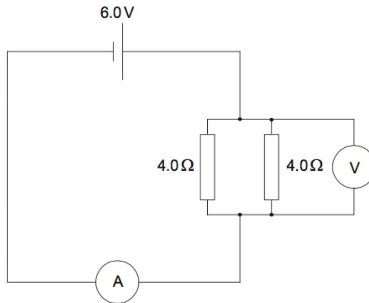
The ammeter has resistance equal to  $1.0\Omega$  and the voltmeter is ideal. What are the readings of the ammeter and the voltmeter?
