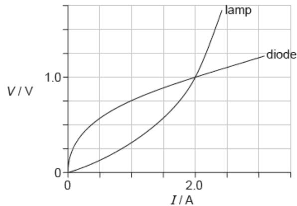
What is the resistance of the lamp and the resistance of the diode when the current in each device is 2.0 A?
