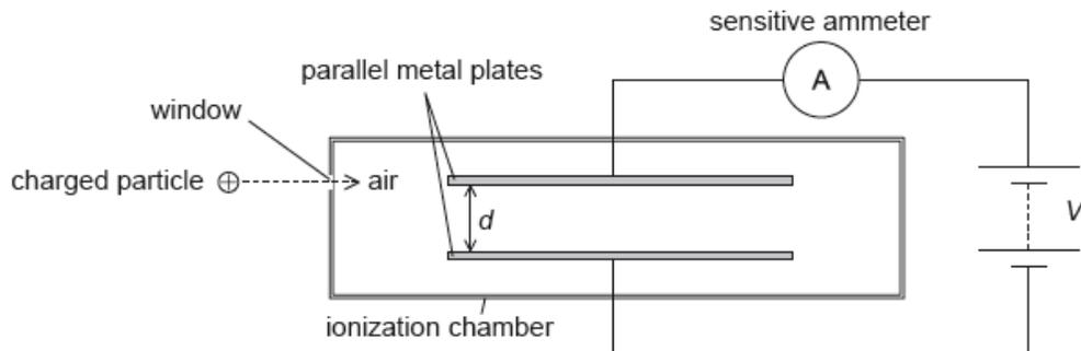
The charged particles enter the chamber through a thin window. They then ionize the air between the parallel metal plates. The ionization of the air between the plates creates an electric field that causes the ions to move towards the plates. Charge now flows around the circuit and a current is detected by the sensitive ammeter.
