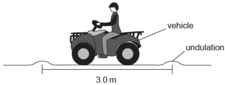
The farmer's seat is mounted on a spring. The system, consisting of the mass of the farmer and the spring, has a natural frequency of vibration of 1.9 Hz.
