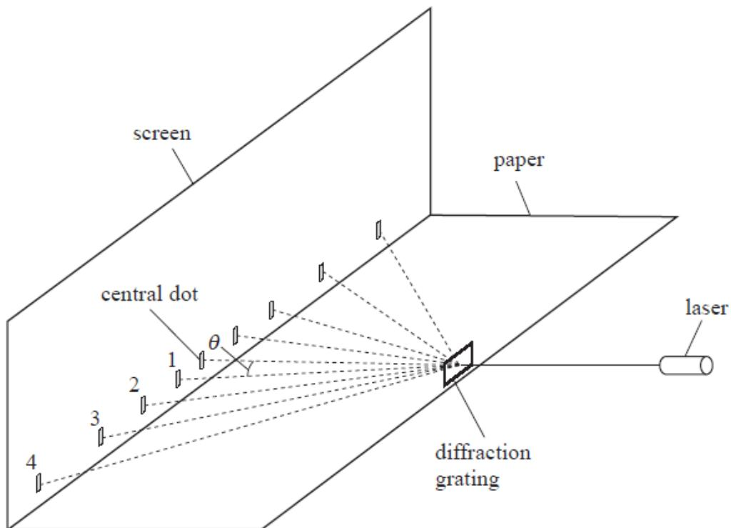
A laser light beam was shone at a diffraction grating. A series of dots of light was produced on a screen. The angles  $\theta$  between the light ray to the central dot and the light rays to the dots labelled 1 to 4 were measured with a protractor.
