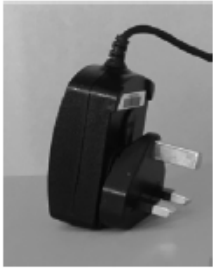
original charging plug 1A, 5V
