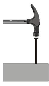
The mass of the hammer is 0.75 kg and its velocity, just before it hits the nail, is 15.0 m/s downward. After hitting the nail, the hammer remains in contact with it for 0.1 s. After this time both the hammer and the nail have stopped moving.
