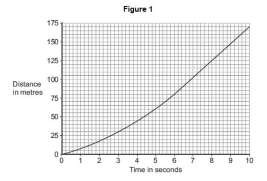
Use Figure 1 to calculate the maximum speed the car was travelling at. Show clearly how you work out your answer.
