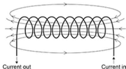
*field lines going through and around coil*
