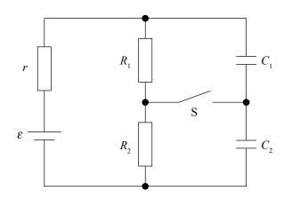
(b) What values do the current in the circuit and charges  $Q_1$  and  $Q_2$  take if the switch is closed and a new steady state is reached?
