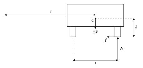
In the diagram, m = mass of the SUV, g = acceleration due to gravity, f = total frictional force on the two outside wheels, N = total normal force on the two outside wheels, C = centre of gravity of the SUV, t = track width, h = height of the centre of gravity, and the radius of the curve is r.
