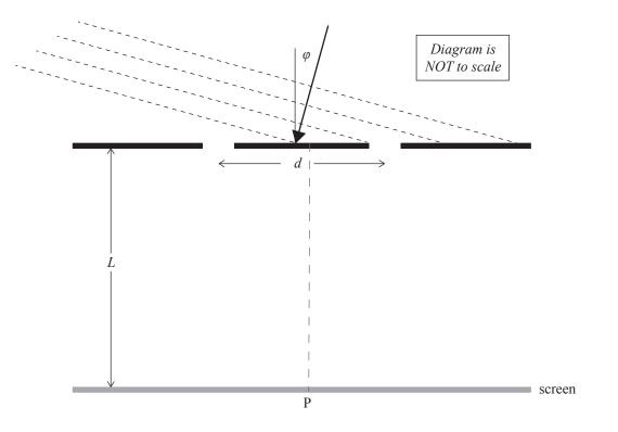
If  $d = 1.00 \times 10^{-4}$  m, and the wavelength is 633 nm, calculate the smallest angle  $\varphi$  that will give an intensity of zero at the point P on the screen as shown in the diagram.
