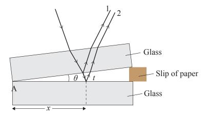
(c) From directly above the position marked A on the diagram, a dark fringe is observed.
