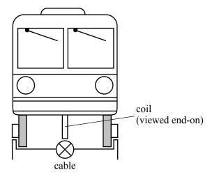
It is suggested that the force between a loop and a long current-carrying wire could be used in the design of a magnetically levitated train (Maglev). Many loops (a coil) are placed vertically in each carriage directly above a cable fixed to the track bed. If the dimensions are chosen so that a >> d and N is the number of loops in a coil then the force produced will be given by:
