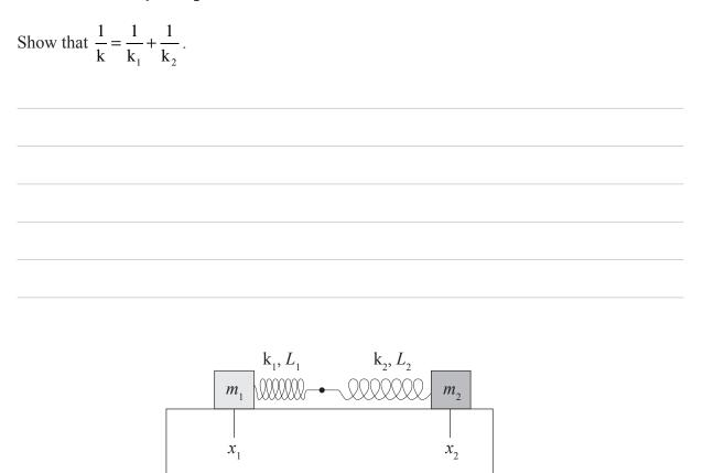
Consider the situation shown above with two springs of spring constants  $k_1$  and  $k_2$  connected together and linking masses  $m_1$  and  $m_2$ , which sit on a frictionless surface. The equilibrium lengths of the springs are  $L_1$  and  $L_2$ , respectively, and the centre of mass of  $m_1$  lies at  $x_1$  and the centre of mass of  $m_2$  lies at  $x_2$ .
