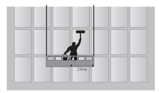
A window-washing cradle of width 4.0 m is suspended from two cables of equal length.
