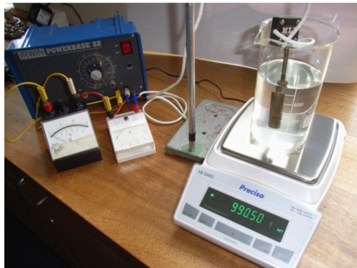
Figure 4. Electrical heater suspended in liquid nitrogen
